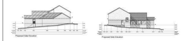
It is proposed to construct the building in a mix of facing brick and render with a reconstituted slate roof. Windows will be manufactured in white upvo and doors in colour coated aluminium (white). Reconstituted stone will be used for all cills.
