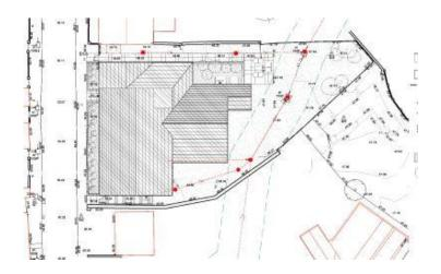
The boundary walls on either side of the site will be retained, as will the palisade fence to the rear, and rear side boundaries. To provide privacy for both future occupants and neighbours, 2.1m high close boarded timber fencing will be erected inside the existing palisade fencing. Landscaping will be provided to front and rear of the building.
